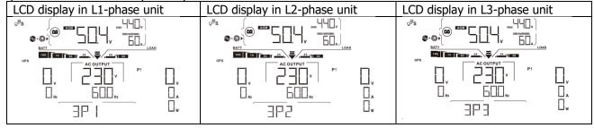
Step 4: Switch on all AC breakers of Line wires in AC input. If AC connection is detected and three phases are matched with unit setting, they will work normally. Otherwise, the AC icon  $\stackrel{\bigcirc}{\bigcirc}$  will flash and they will not work in line mode.
