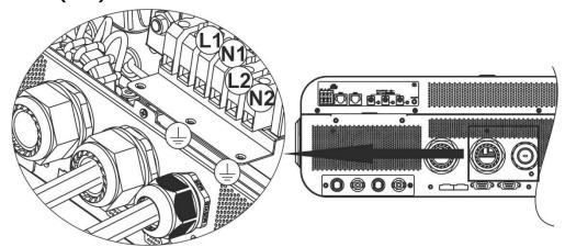
2. Make sure the wires are securely connected.
