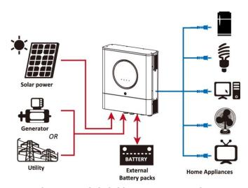
Figure 1 Basic hybrid PV System Overview
